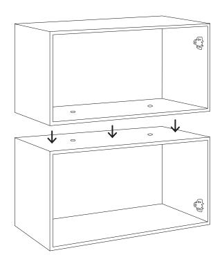
**1.** Place the two modules on top of each other so that the sides with the two holes face each other in the middle.
