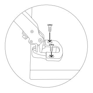
**3.** Place the overlay hinges (door hinges) into the cut-outs in the doors as shown in the illustration and secure them with the screws.
