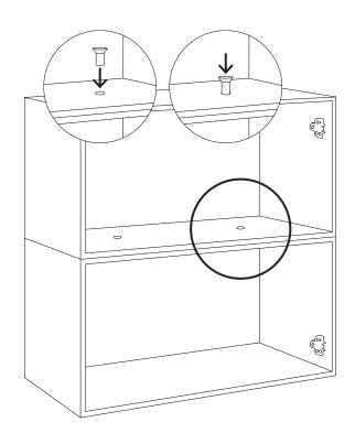
**2.** Insert the supplied pins into the holes.
